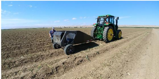
development of the robotic asparagus harvester. Hin and his team, along with Robotics Plus, are developing version 1.5 of the harvester with the aim of improving spear cutting. The latest version is three times faster than the first harvester and trials are planned at Boyds Asparagus in the Waikato in September. The team plan to be able to demonstrate it by the end of October, so watch this space for more on this exciting development.
